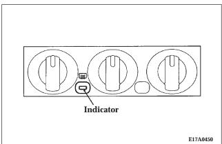
The electric rear window defogger can be operated when the ignition key is in the "ON" position.
